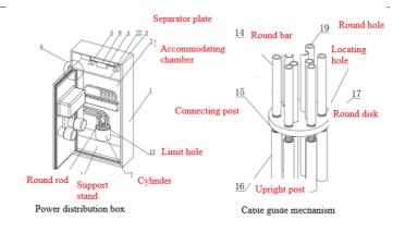
The petitioner believes that D2 discloses a power distribution cabinet, wherein a concentrator 6 (cylinder body 61 + wire clamping slot 62 + fastener 63 + venthole 64; see the Figure below) may be placed on a cable that needs to be mounted, and the structure thereof is also cylindrical. Thus, the petitioner believes that "the concentrator" disclosed in D2 is equivalent to "a cable quide mechanism" in the patent involved.
